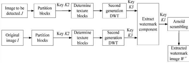
Figure 2. Digital watermark extracting algorithm flowchart
