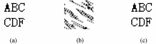
Figure 4. (a) Original watermark. (b) Scrambling watermark when  $K_1=5$ . (c) Extracted watermark
