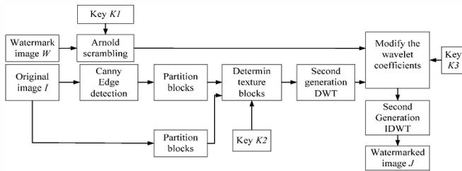
Figure 1. Digital watermark embedding algorithm flowchart
