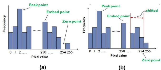
Fig. 2. Example of histogram before and after shifting the pixels in our proposed scheme: (a) Histogram before shifting with peak point = 2, embed point = 250 and zero point = 254; (b) Histogram after shifting the pixels.
