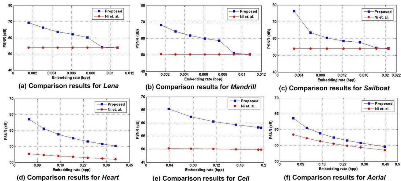
Fig. 4. Capacity vs. distortion characteristics comparison results for six different images.
