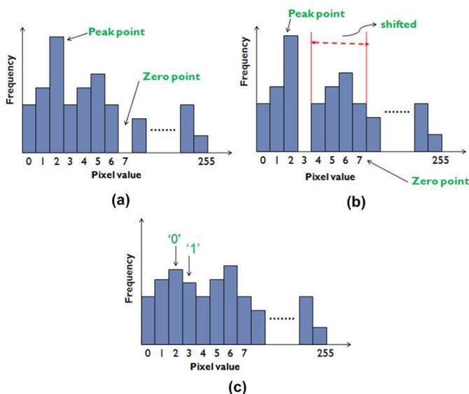
Fig. 1. Histogram bin shifting proposed by Ni. et. al [2]. (a) Histogram before shifting with peak point = 2 and zero point = 7; (b) Histogram after shifting the pixels; (c) histogram after watermark embedding.
