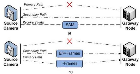
Figure 7. Path switchover in case of path breakdown.
