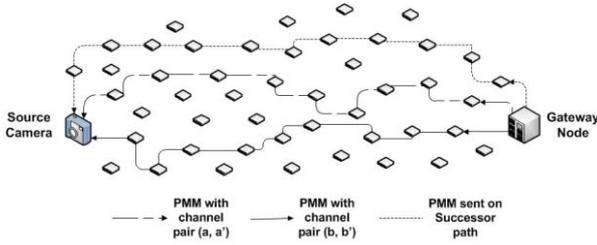
Figure 4. The flow of PMM sent by the gateway along the selected paths.
