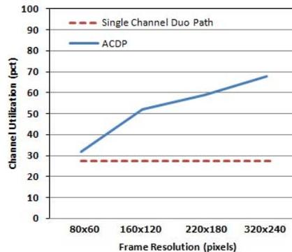
Figure 11. Channel utilization with different frame resolution.
