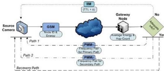
Figure 5. The flow of control packet exchange during path selection of Stage I.
