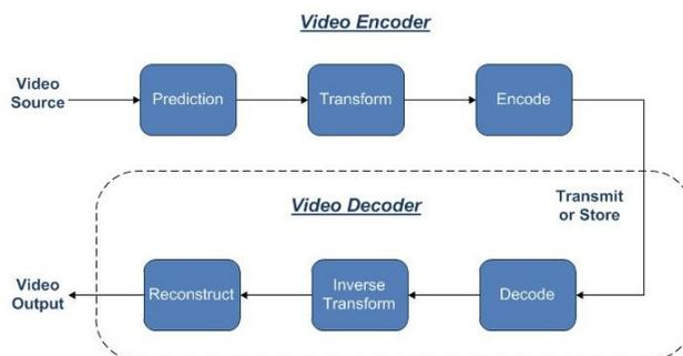
Figure 1. The H.264 video encoding and decoding process.
